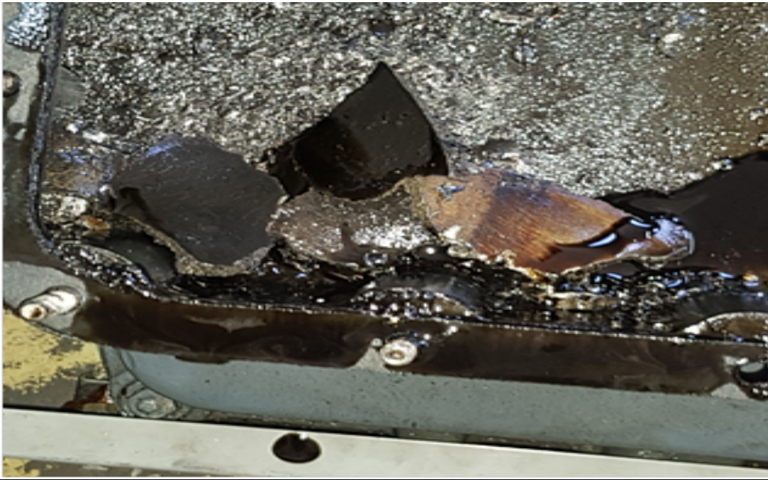
Figure 2d: Oil sump with metal debris of all sizes
