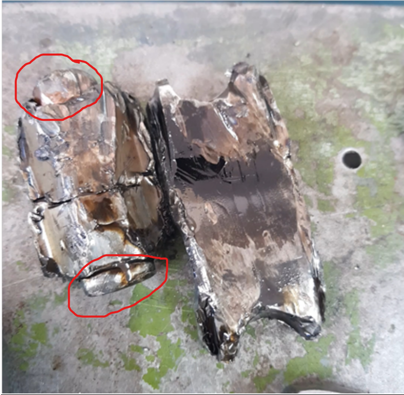
Figure 3b: Broken off big end connecting rod cap (Note that the connecting rod bolt and nut are still intact)
