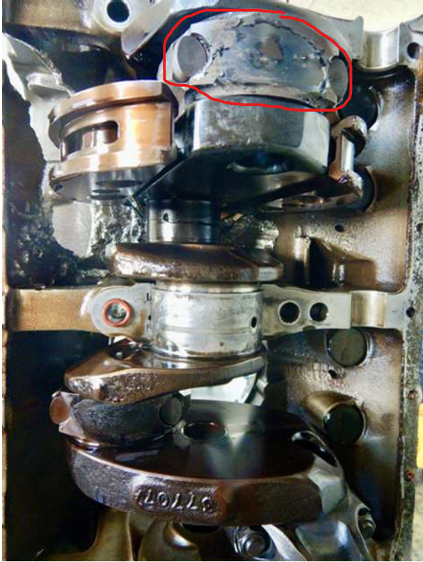
Figure 6a: Evidence of severe heat damage
