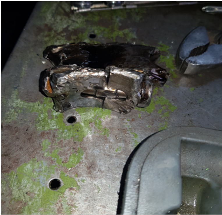
Figure 3a: Broken off connecting rod big end cap
