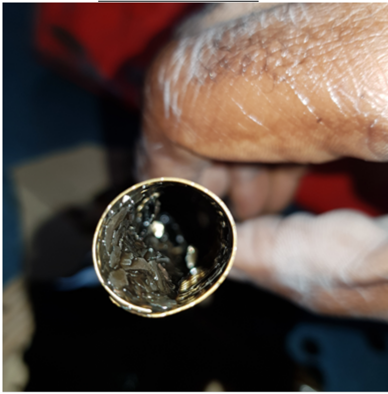
Figure 2bb: Main oil filter canister cut open and exhibiting dried up sludge of oil and some metal debris
