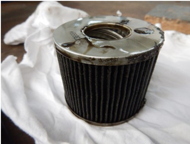
Figure 2a: Main oil filter removed from the canister during lab testing
