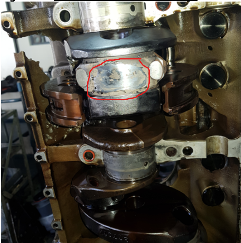
Figure 6a: Evidence of severe heat damage
