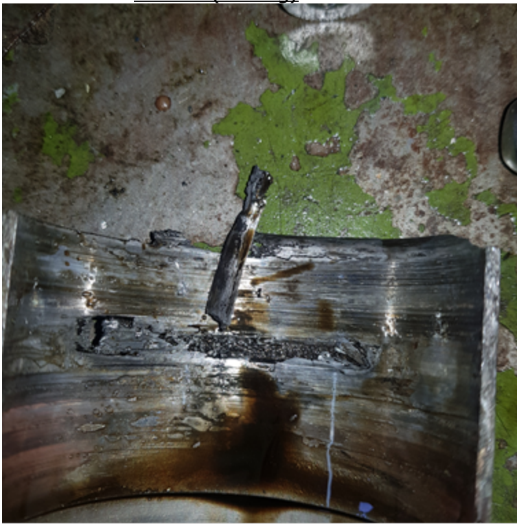
Figure 5b: Metal debris of broken main bearing
