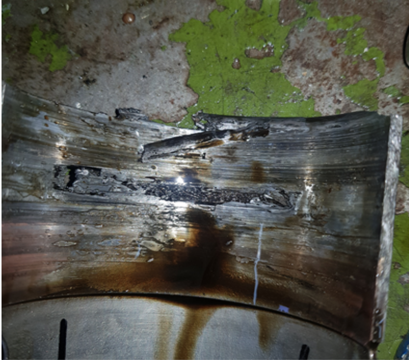
Figure 5a: Main bearing with broken metal pieces due to metal on metal contact (chafing)
