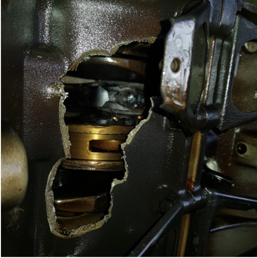
Figure 3d: Crankcase bottom side punched out by uncontained connecting rod
