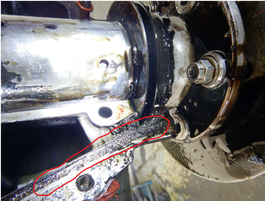
Figure 4a: Sludge made up of metal debris and rubber material collected in the annul
